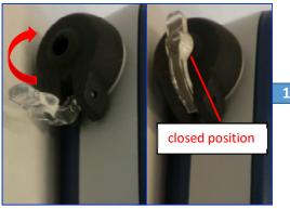
1. Place the self-checkstandard in the closed position (i.e. flip the self-checkstandard up and insert it into the nose cone).
