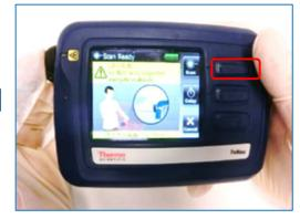
3. The *Scan Ready* screen appears. In this screen, select the "Scan" option again by pressing the key next to it.
