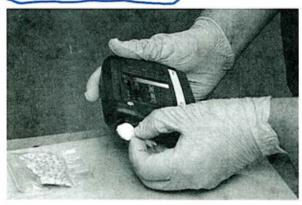
The TruNarc analyzer can scan suspected narcotics through a sealed plastic bag in seconds.
