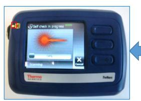
4. The laser light glows indicating that the laser is active and analyser is performing the scan.
