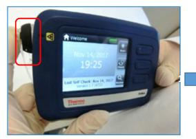
1. Ensure that the self-check standard is in the open position. Hold the scoop end of the test kit against the nose cone of the analyser to scan the metal wafer. The cup of the scoop should be centered over the opening of the nose cone. Use the forefinger to firmly press against the nose cone.
