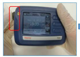
1. Self-check standard should be in the open position. Press the packet of sample firmly against the nose cone of the analyser. Ensure the laser sample point (i.e. 2 mm away from nose cone) is positioned at the sample inside the packet.
