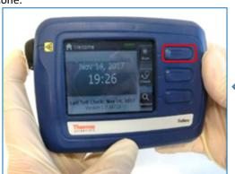
3. When the test kit is in the correct position, select the "Scan" option in the *Welcome* screen by pressing the key next to it.
