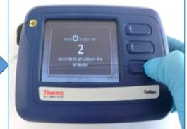
2. After holding for 5 seconds, the analyser will begin a 5 seconds countdown and the analyser will be turned off after 5 seconds.
