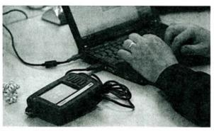
Test records in TruNarc's tamper-proof system can be transferred to a PC, reducing the administrative burden of maintaining the chain of custody of samples and evidence.
