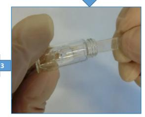
Insert the scoop containing the sample into the vial and stir gently to dissolve the sample. Ensure the filled scoop is fully submerged in the ethanol solution.
