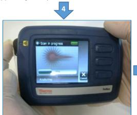
5.When the laser indicator light turns off, the analysis screen appears. The test kit can now be move away from the nose cone.
