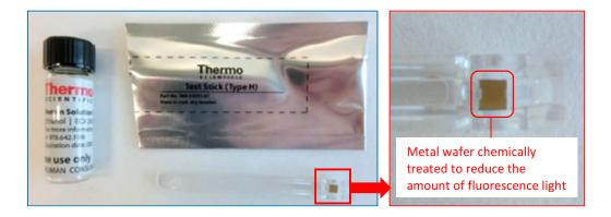
Fig. 9: Components of a Type H test kit
