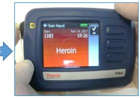
6. When the analysis step completes, the analyser display a result in the *Scan Result* screen. Select "OK" to return to the *Welcome* screen.
