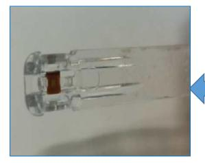
4. Remove the test stick and shake it in the air to allow the ethanol to evaporate.A thin film of dried sample will be coated on the metal wafer at the base of the scoop.
