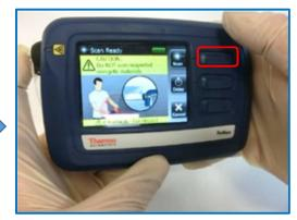
2.The *Scan Ready* screen appears. In this screen, select the "Scan" option again by pressing the key next to it.
