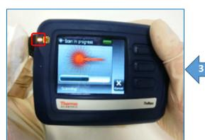
5. The laser light glows indicating the laser is active and the analyser scanning. Hold the sample <u>still</u> during the scan to avoid moving the sample during the scan.
