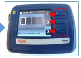
2. The *Activate Laser* screen appears. Enter the laser activation code by pressing the button next to each number.
