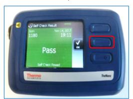
5. The result of the check will appear in the *Self-check Result* screen after a few seconds.
