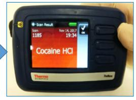
4. The analyser will display a result in the *Scan Result* screen. Select "OK" to return to the *Welcome* screen.
