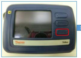
1. Press and release the bottom key on the TruNarc analyser.
