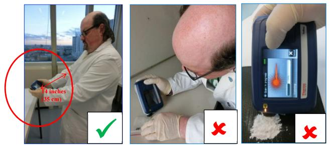
Fig. 4: Safety distance from nose cone of analyser when scanning is performed
