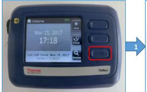
1. Press and hold the bottom key or 10 seconds.
