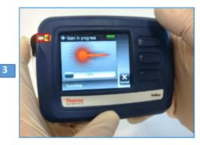
4. The laser light glows in a few seconds indicating that the laser is active and the analyser is performing the scan. Hold the test kit on the nose cone until the laser light turns off.
