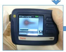
6. When the laser indicator light turns off, the analysis screen appears. The packet can now be move away from the nose cone.
